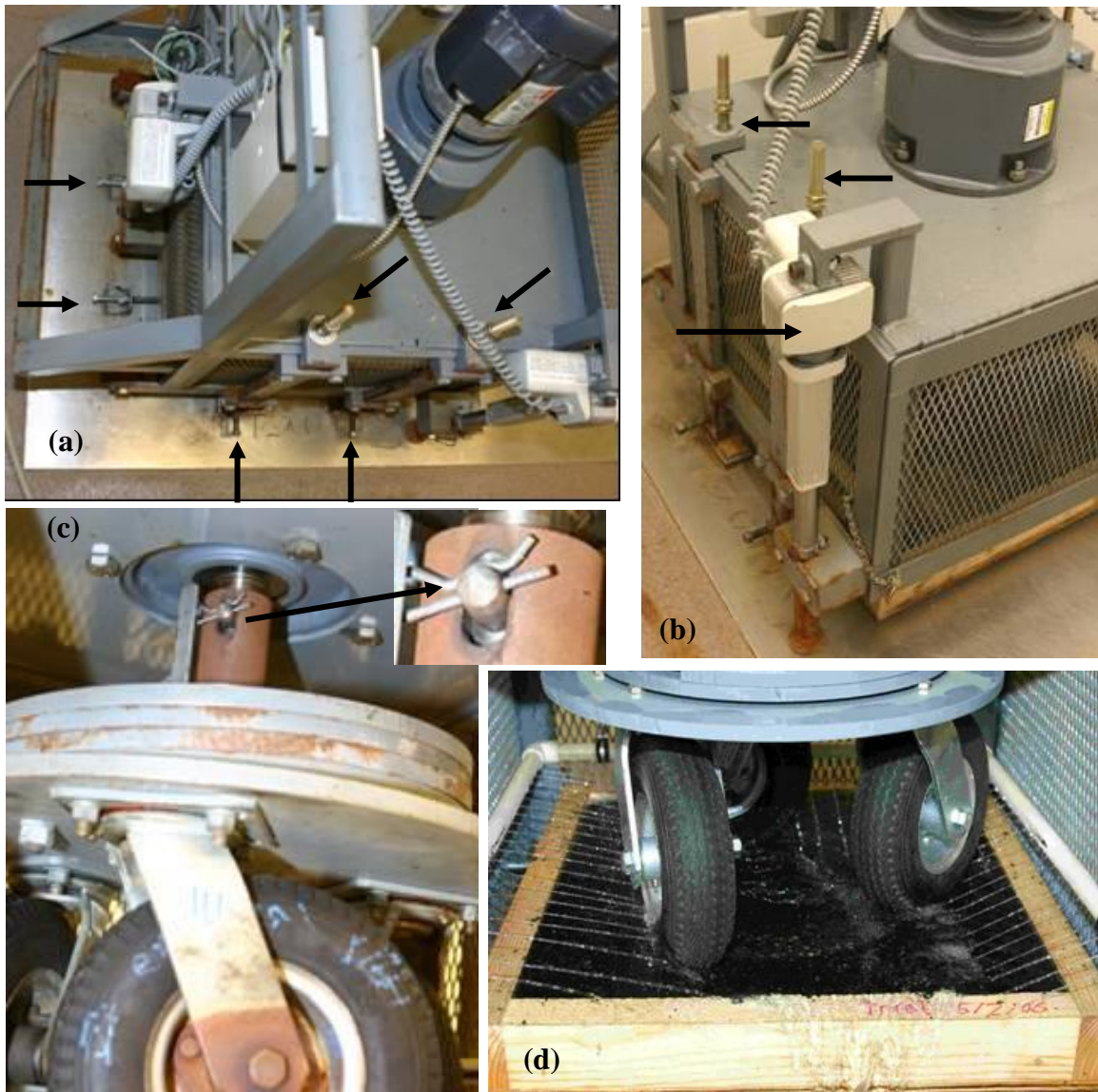
Figure 18. Details of the CTPM device: (a) alignment and level device, (b) level device and actuator, (c) force control bolt and (d) rubbers washed with water
