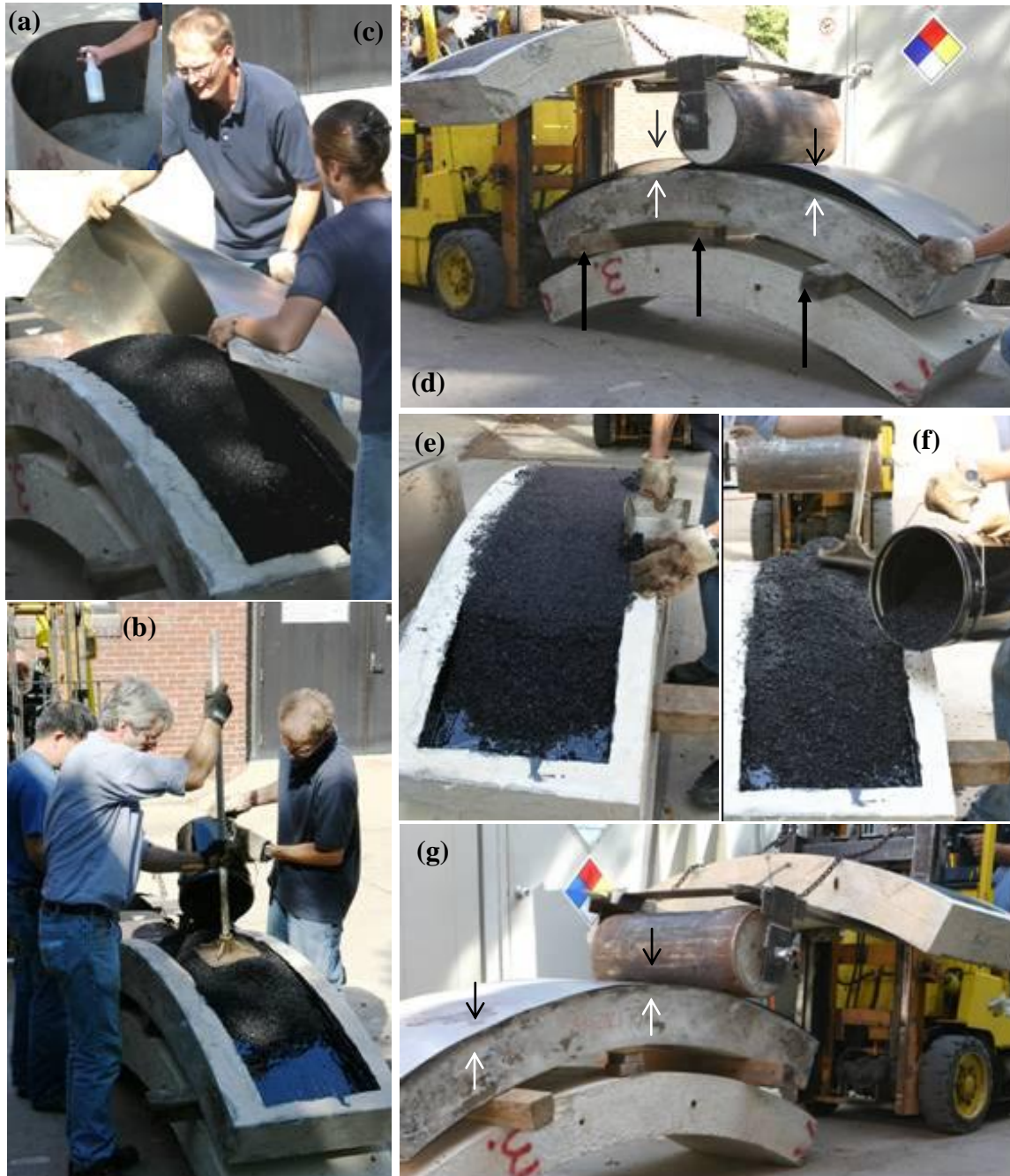
Figure G 4. . Stages of the TPTA segments compaction process: (a) spraying thin metal sheet with an anti-adhesive agent, (b) first stage: pre-densification, (c) specimen before the first stage of compaction, (d) first stage: compaction, (e) removing mixture covering top of the walls, (f) second stage: pre-densification and (g) second stage: compaction
