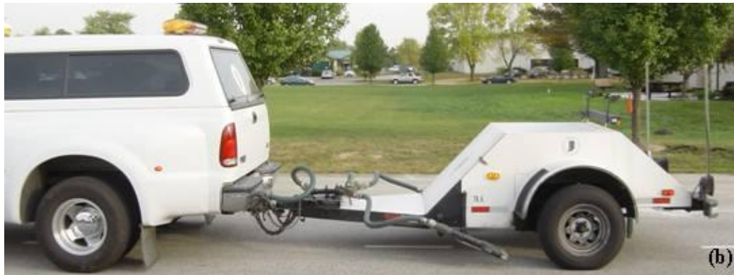
Figure 21. ASTM E-274 towed friction trailer: (a) oblique and (b) side views
