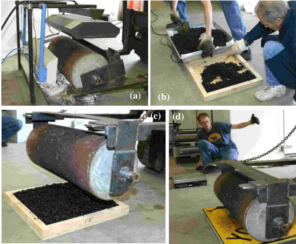
Figure 15. Stages of the friction slab compaction process: (a) preheating roller, (b) mix placing and pre-densification, (c) initial compaction and (d) final compaction
